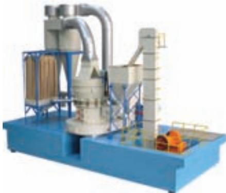
After this, the ground stuff are carried by the air from the blower into the separator for screening. The fine powers are blow into the cyclone collector and are poured out through the output-powder valve as the final products and the rough stuff after the screening will be recycled back into the grinding chamber for regrinding. The set's airflow system is closely sealed up and circulated under condition of negative and positive pressure.
