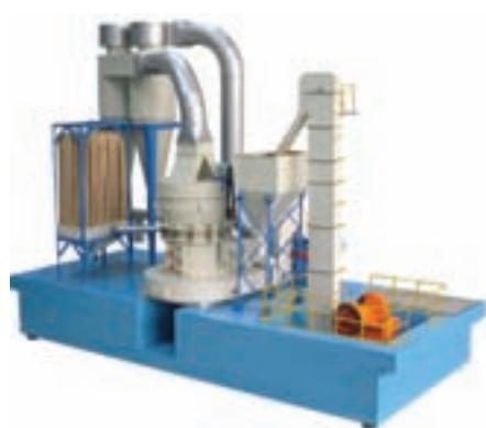
After this, the ground stuff are carried by the air from the blower into the separator for screening. The fine powers are blow into the cyclone collector and are poured out through the output-powder valve as the final products and the rough stuff after the screening will be recycled back into the grinding chamber for regrounding. The set's airflow system is closely sealed up and circulated under condition of negative and positive pressure.
